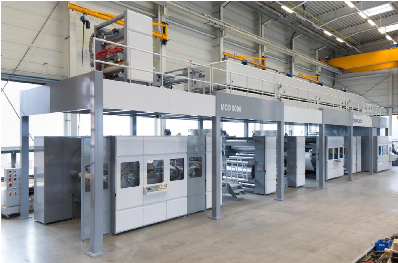
The complete coating line – MCO500
