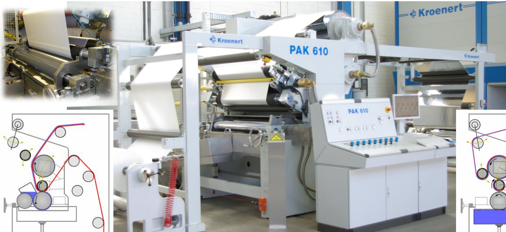
Hotmelt feeding by dipping for low viscos coating materials
